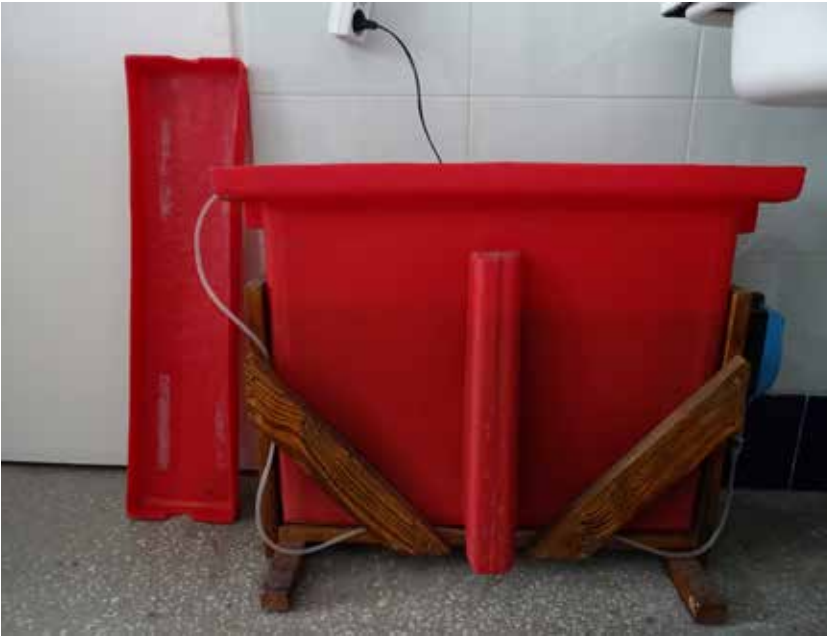
Pionowa kufeta z aeratorem do trawienia matryc miedzianych w chlorku żelaza Vertical etching tank with aerator for etching copper matrices in iron chloride
